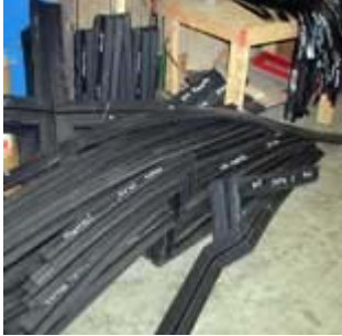
Rubber sealing components are also factory-fabricated for crosses, tees, upturns, and curbs. All welds are reinforced with Santoprene thermo-plastic rubber sheet for durability.
